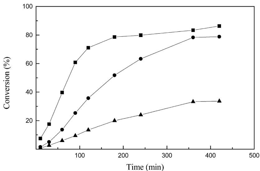
**Figure 7.** Bioconversion profile of 6-bromo- $\beta$ -tetralone to 6-bromo- $\beta$ -tetralol using methoxyethanol as the solvent with an initial reactant concentration of 1 g/L (■), 5 g/L (●), and 10 g/L (▲).
