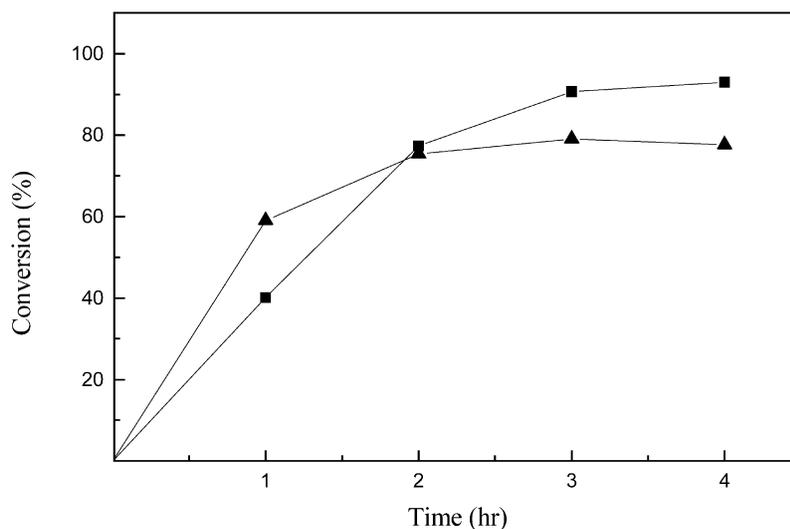
**Figure 9.** Bioconversion profile for a first (■) and second batch (▲), where the product and remaining reactant have been separated from the enzymes and cofactors, which have already completed a first batch reaction.
